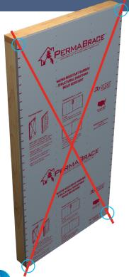
DO NOT fasten the four corners first. In order to prevent gaps or rippling, it's important to move horizontally, from one side of the panel to the other, when installing.
