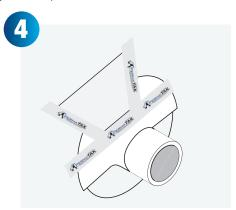
Tape over the 45° cuts using PermaTak® Flashing Tape.
